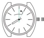
Pull out the crown, and set the time. If your watch is one whose crown cannot be pulled out (a screw-lock type crown), turn the crown counterclockwise to loosen the screw and then pull out the crown and set the time.
