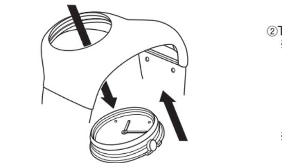
When setting the watch unit to the Ti body, fit the crown position to a notch on the back of the Ti body.
